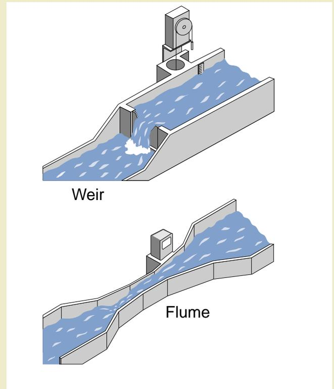
Figure 17 – Typical weir/flume configurations
