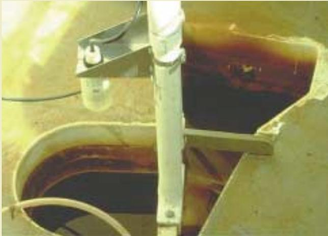
Figure 18 – Ultrasonic sensor
