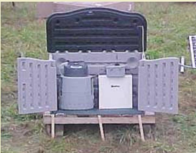
*Figure 14 – Data retrieval using a cellular modem*
