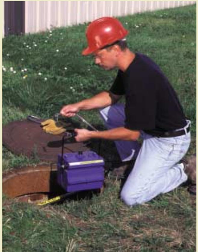
Figure 21 – Isco 2150 Area Velocity Module on site
