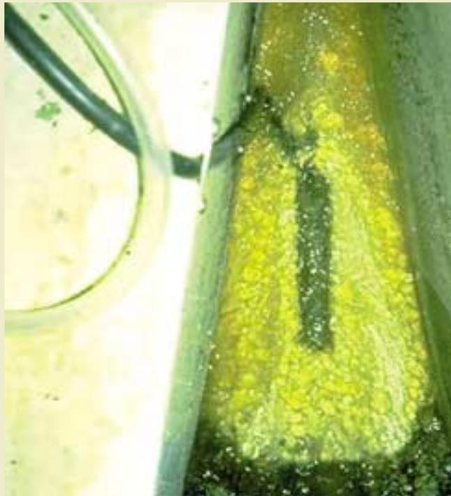
Figure 19 – Submerged pressure transducer in flow stream
