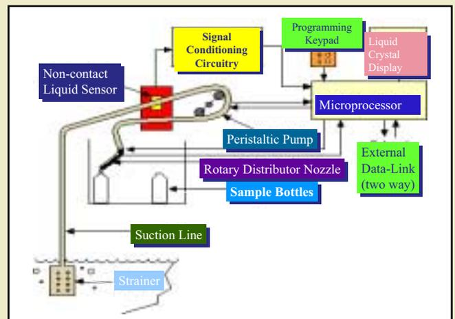
Figure 7 – Typical sampler schematic
