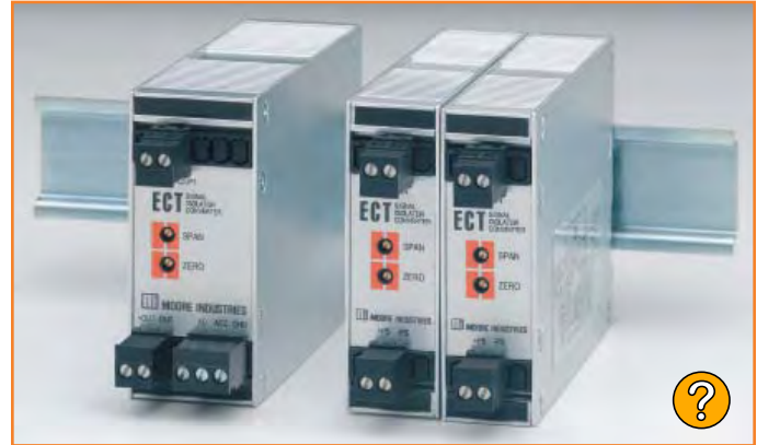
Figure 20. Solid aluminum housings designed with no openings, covered mounting holes and no exposed circuit boards help block RFI/EMI noise.
