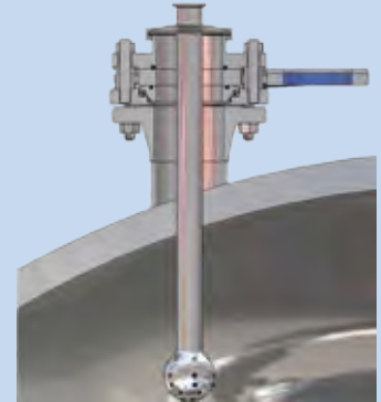
Sprayball = No Additional Nozzle Needed
