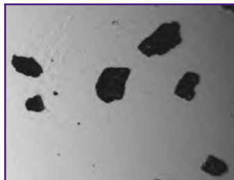
Raw image of stone in RockSizer™
